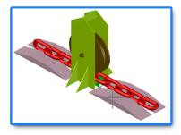
Hence CubicWheels Engineered and installed a roller arrangement with box frame with overall size of (5.5m Width x 2.650m Height) at the stern side of material barge in order to facilitate the lay down of mooring chain into the sea bed without any twist. This roller arrangement proved to be very conducive and less expensive method for chain laying process.
